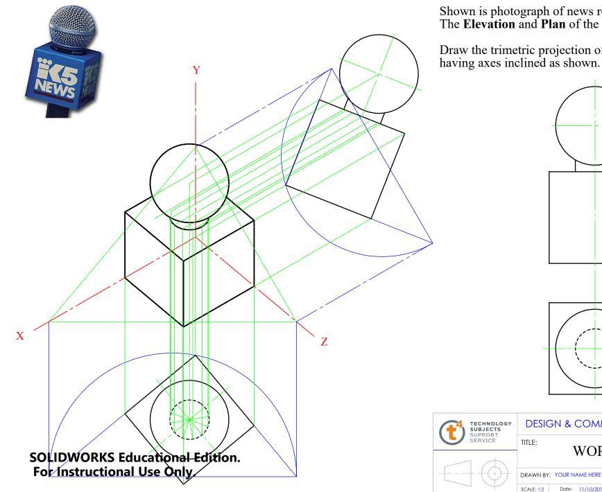
Shown is photograph of news reporters microphone. The **Elevation** and **Plan** of the microphone is shown.
